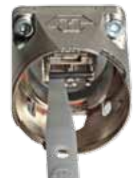
Exchange of SFP module Release and pull SFP module
