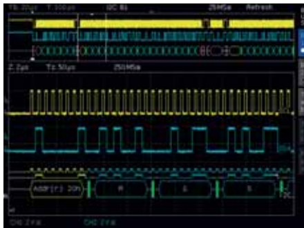
SPI bus signal, MISO / MOSI decoded
