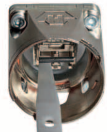
Exchange of SFP module Release and pull SFP module
